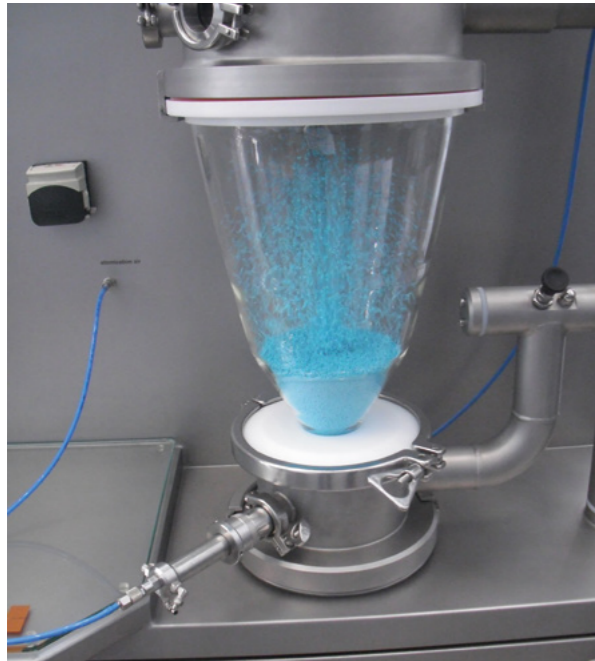
↑ Spouted bed coating in the laboratory processes
