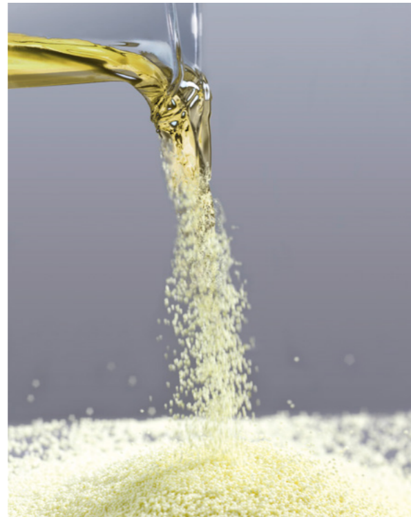
↑ In the fluidized bed, liquids can be converted into dry granules
